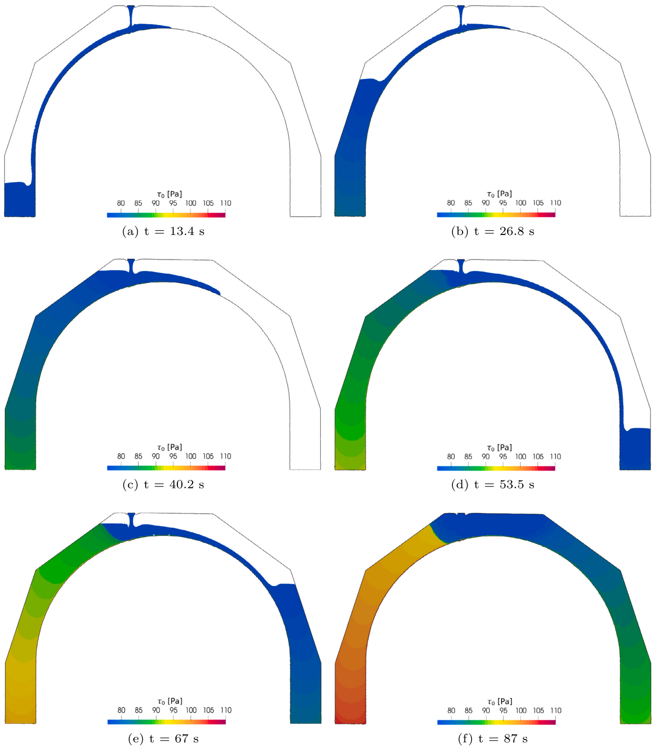
Fig. 9. Static yield stress distribution at different times (a–f) of the 2D process of filling of the mould.
