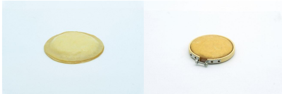
Figure 4. On the left: Sample made of two layers of BC with cotton fibers padding, made with exsitu method; On the right: sample inserted in wood drum for the tensioning.
