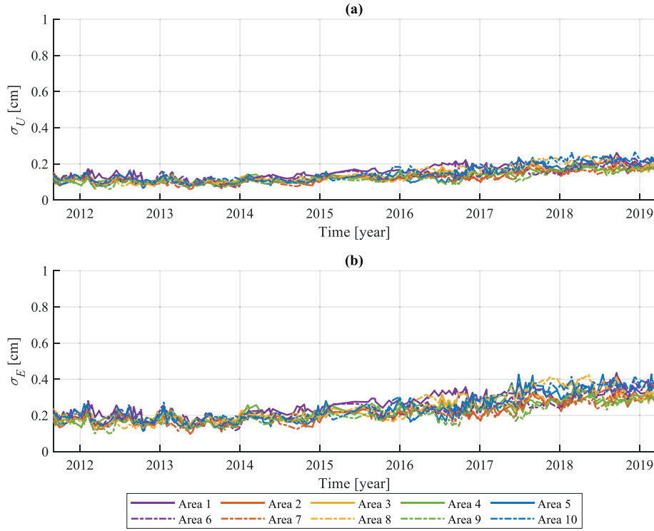
Fig. 19. Error of the reconstructed structural displacements using a tailored grid, removing PSs outside the bridge: (a) Vertical and (b) Longitudinal.
