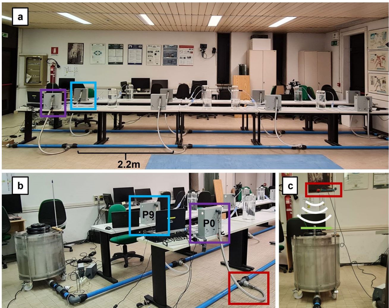
Fig. 6 a MEV functional prototype tested via patient simulators. Each PCU is separated by 2.2-m modules. A linear “U” layout was tested to check the ventilation quality at the most distal patient (P0—purple rectangle). b BJS and initial part of the BPD, the most proximal patient (P9—blue rectangle). c Ultrasound detector of BJS bell height
