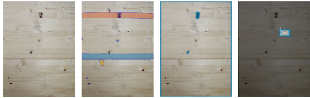
Figure 6. From the left: original image; mask prediction with the “everything” function; mask prediction with bounding box corresponding to the size of the image; mask prediction with bounding box corresponding to a specific wood knot.
