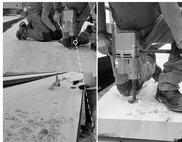
Figure 1. Traditional manual defect removal process in glulam beams, as currently practiced in industrial wood lamination production. The images illustrate the high physical demand due to the operators' working posture, as well as the significant mental effort required to maintain prolonged concentration for accurate detection and removal of knots. Additionally, continuous manual control of the router's rotation adds to operator fatigue and task complexity.
