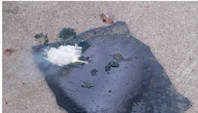
Figure 6 – delamination, ignition of a combustion reaction and fumes in a laser decoating operation
