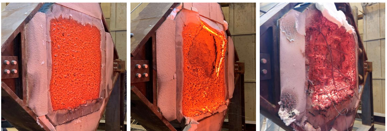
Fig. 9. Specimen SFRC F27 (left), SFRC F03 (center) and R/C F08 (right) as soon as they were extracted from the furnace.
