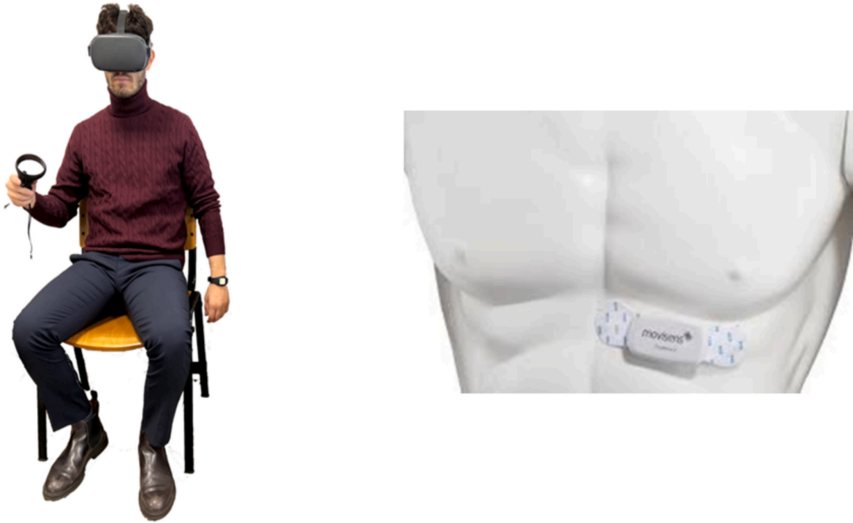
Fig. 1. Left: Volunteer wearing the VR headset, embedding the inertial sensors from which the head ballistocardiography (H-BCG) signals are derived, while starting the protocol in sitting position, Right: representation of the ECGMove4 sensor, attached by two electrodes on the thorax, utilized to acquire the ECG, from which the reference respiratory signal was then obtain, as well as the inertial signals, utilized for synchronization purposes with the H-BCG obtained by the VR headset.
