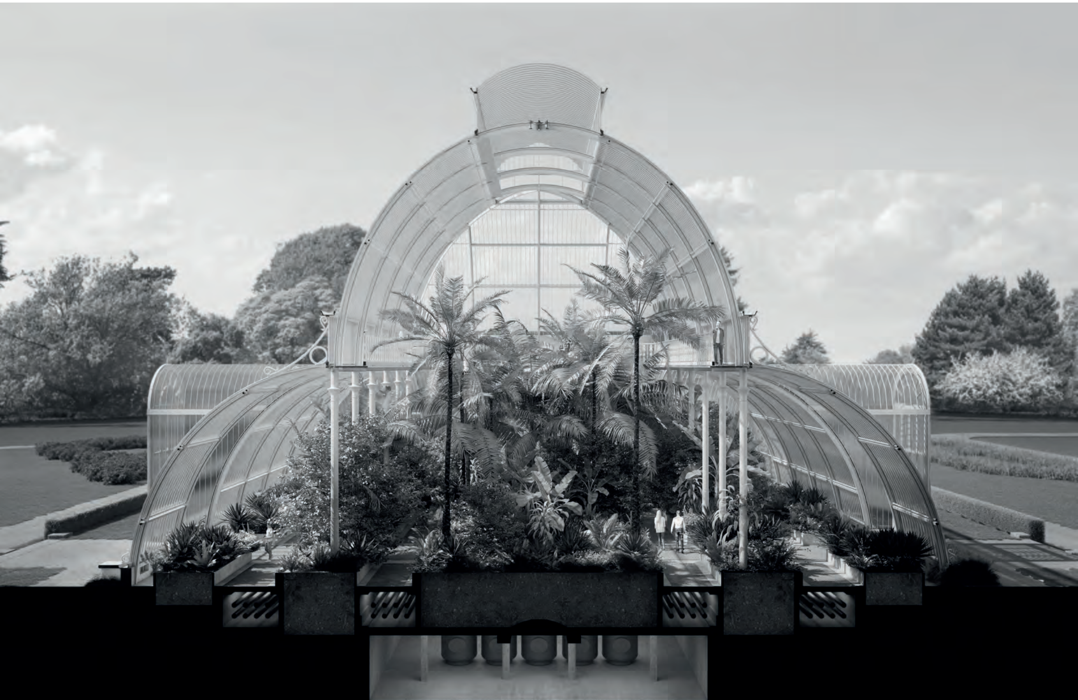
Palm House at Kew Gardens - cross section. Drawing by AHMM, 2022. Credits: @AHMM
