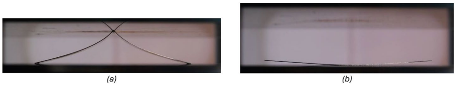
Fig. 3 Sequence of deformation during a flattening test; (a) while flattening the flanges mildly bend upward, (b) after unloading the flanges lift upward, with a springforward phenomenon
