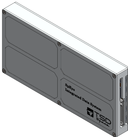
Fig. 4. Computer Aided Design (CAD) representation of the SpEye Free Flyer IDS.
