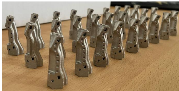
Figure 5: Thruster printed specimens: longitudinal, spiral and zig-zag samples are reported.
