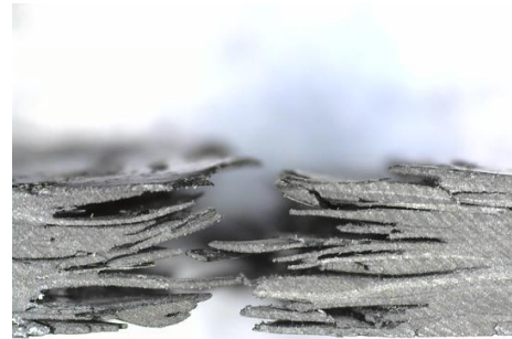
(b) Detail of fiber breakage
