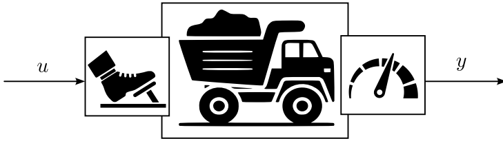
Figure 1.1: A motivating example: cruise control for a truck.
