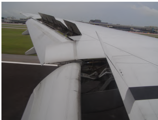
Figure 16.1: Fully extended flap of a Boeing 777 during landing (Creative Commons).
