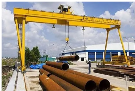
(a) A heavy-duty gantry crane (Creative Commons)
