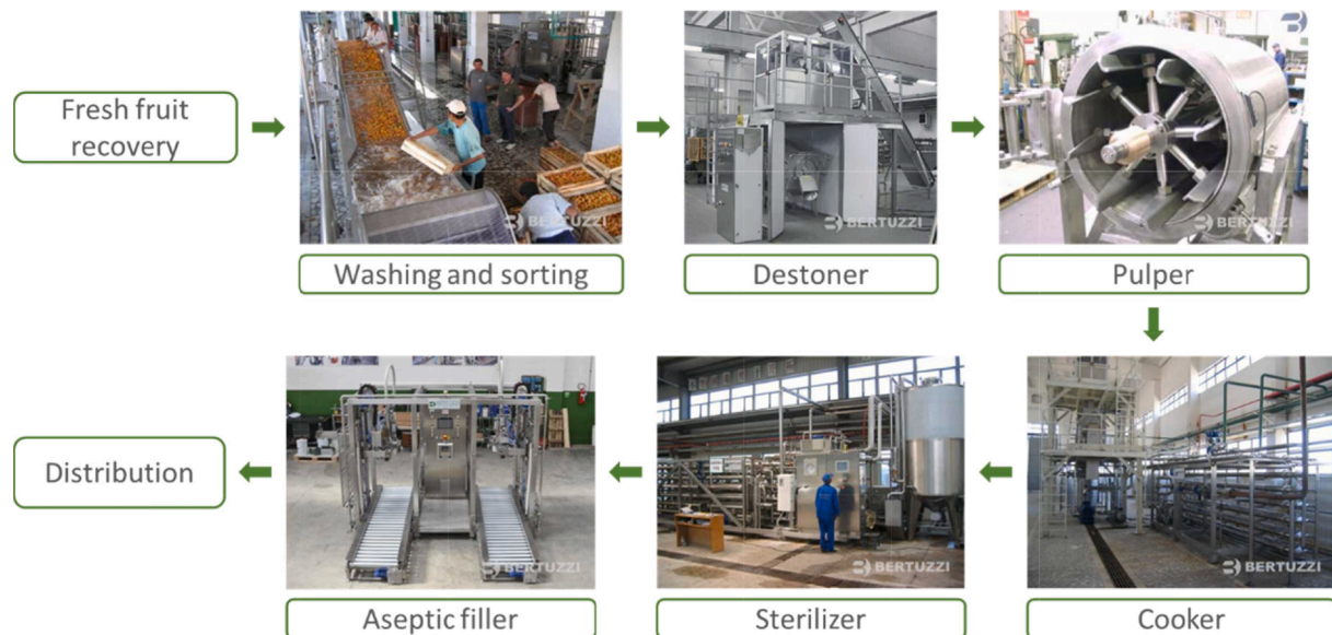
Fig. 7. Schematization of the process line to produce nectarines' puree.
