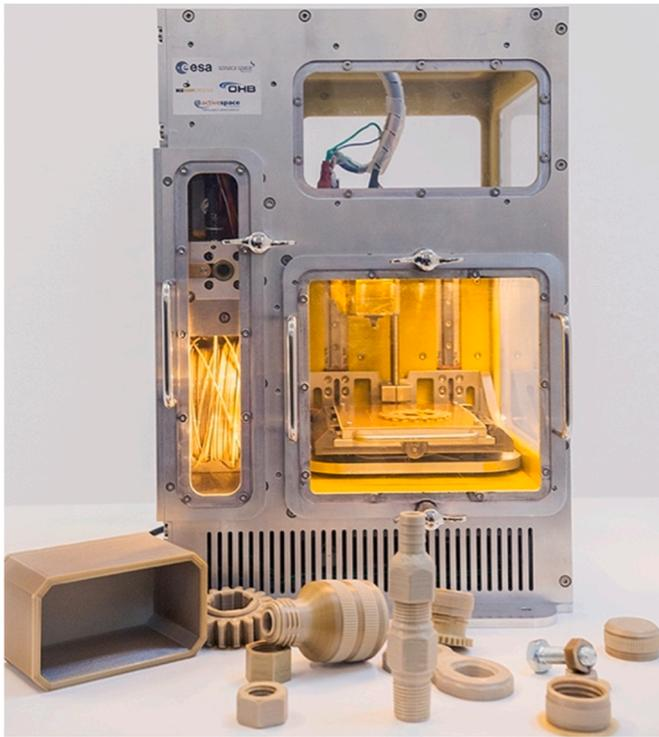
Fig. 12. ESA's Manufacturing of Experimental Layer Technology (MELT) FDM printer [57].
