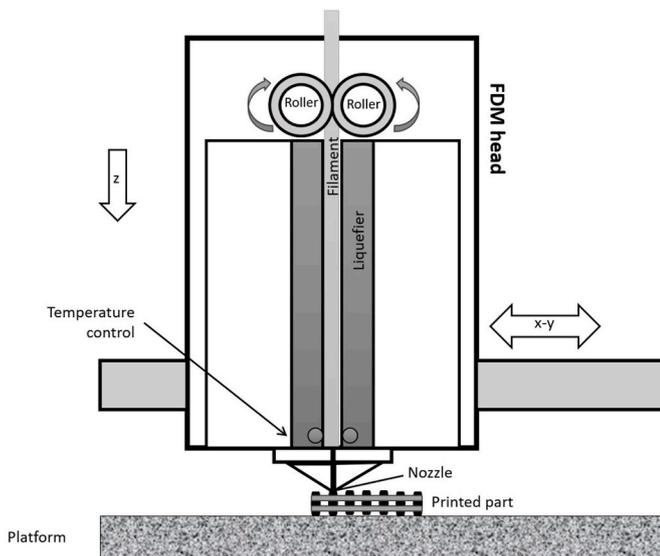
Fig. 8. Schematic of FDM process [64].
