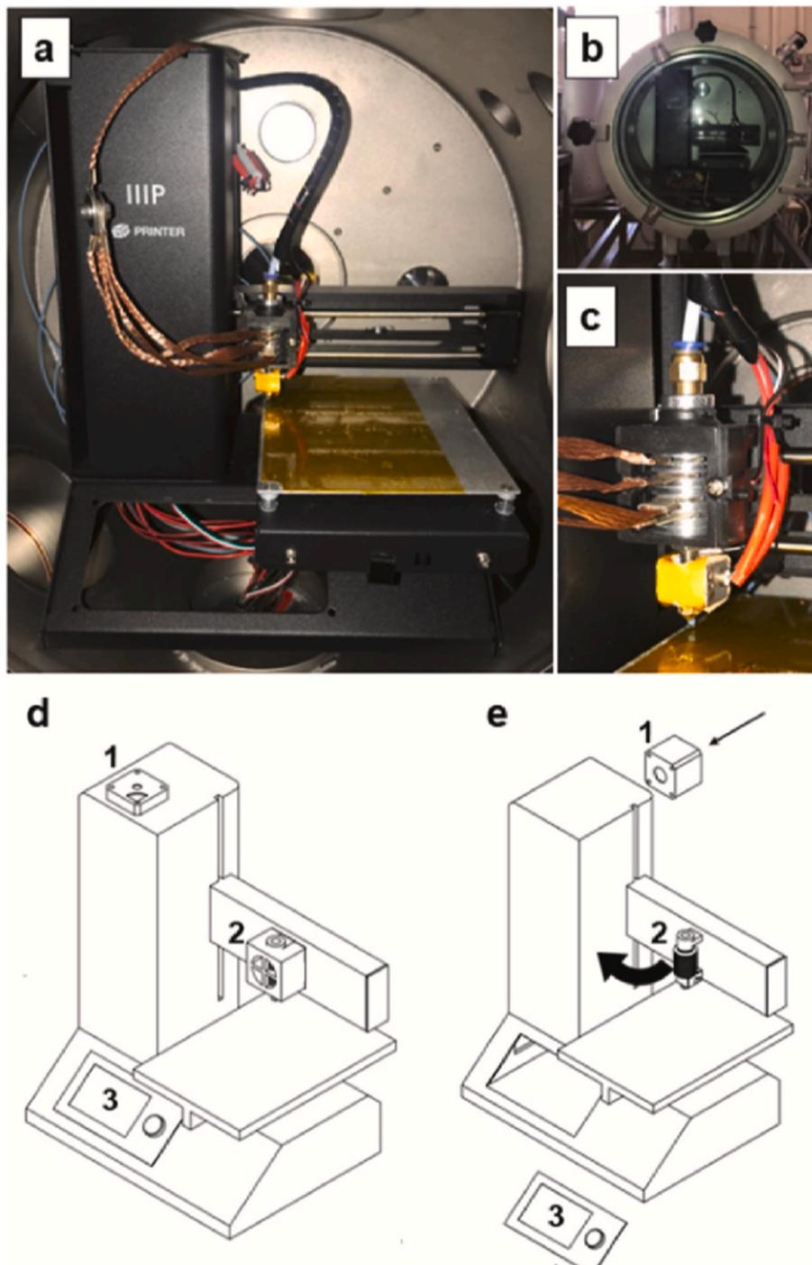
**Fig. 9.** a) Vacuum FDM setup, b) overall view of the setup, c) detail of the reconfigured hot head, d) schematic of FDM device before modification, e) Schematic of FDM device after modification. (1) extruder motor repositioned, (2) installation of copper braids, (3) detaching of the control board [97].
