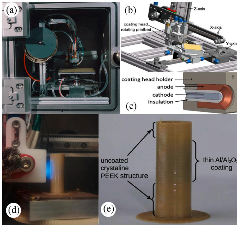
Fig. 13. (a)The FDM device in a vacuum environment, (b) a 3D model of the coating apparatus, (c) a schematic of the vacuum arc coating source, (d) a vacuum arc coating process, (e) a PEEK tube printed and coated with  $Al_2O_3$  [99].
