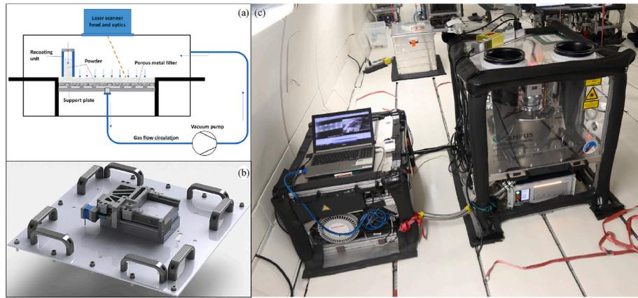
Fig. 7. (a) Schematic of the gas flow-assisted powder deposition; (b) Rendering of the powder deposition unit; (c) Pictures of the LBM unit in microgravity as mounted [85].
