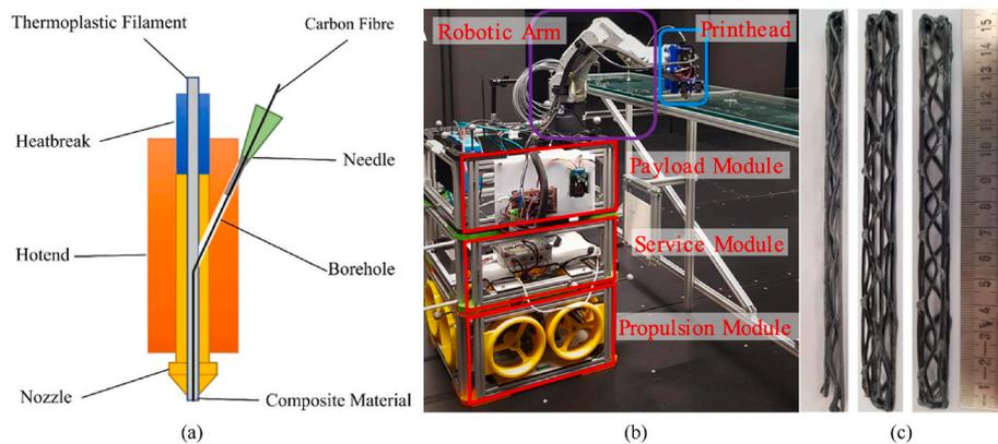
Fig. 15. (a)Schematic of modified FDM printhead, (b)modified FDM device,(c)printed samples [75].
