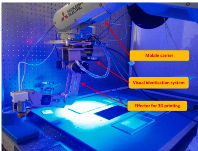
Fig. 17. 3D-printing end-effector on a multi-degree-of-freedom robotic arm [85].
