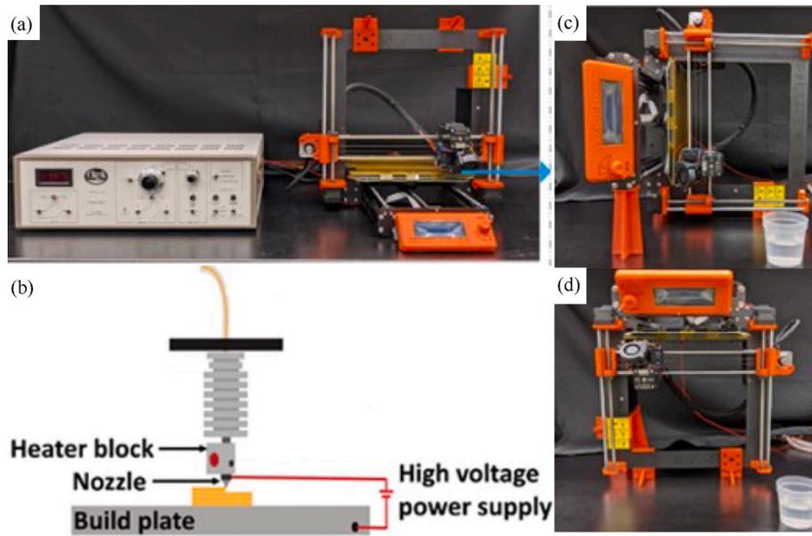
Fig. 16. a)E-FDM device, b)E-FDM schematic diagram, c)E-FDM vertical printing orientation, d)E-FDM reverse printing orientation [100].
