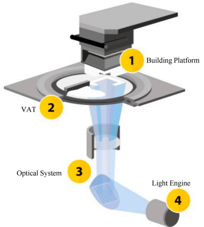
Fig. 18. Schematic of Lithography-based Ceramic Manufacturing [104].
