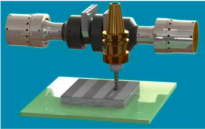
Fig. 22. Ultrasonic Additive Manufacturing unit [72].
