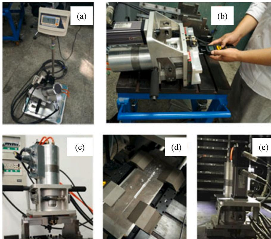
Fig. 20. Portable FSW equipment: (a)Weight measurement, (b)rotary speed test, (c)ground weld test, (d)weld seam, and (e)test in simulated conditions [81].
