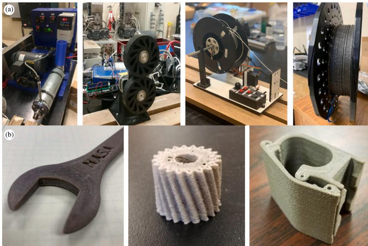
Fig. 14. a) Filament extrusion process, b) Printed basalt-ABS samples [65].
