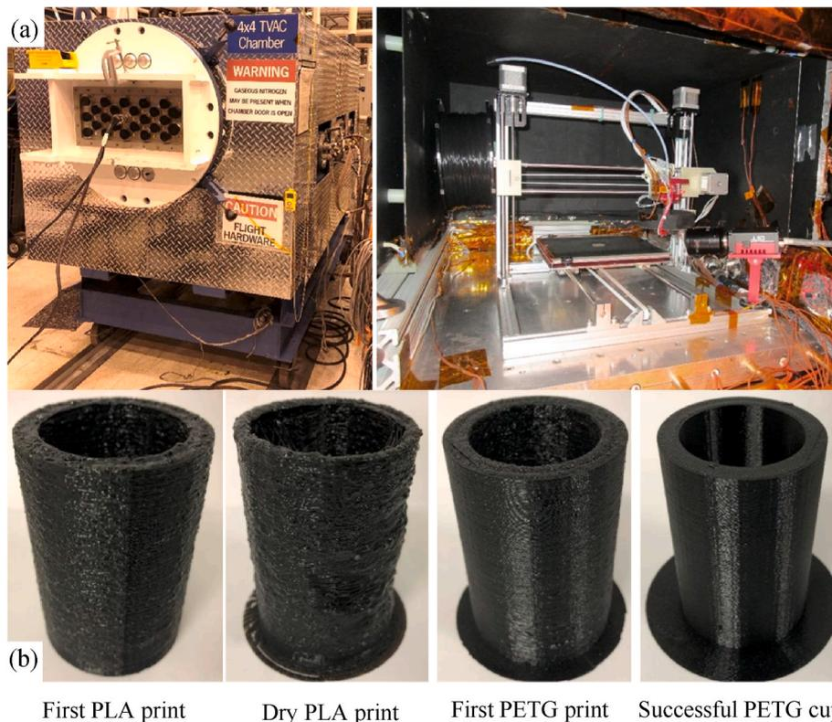
Fig. 10. (a)The modified FDM device was installed in a TVAC chamber, and (b) The cup model prints were completed [98].
