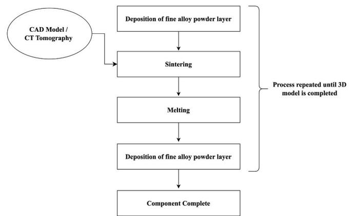
Fig. 6. Stages of LBM (adapted from Ref. [93]).
