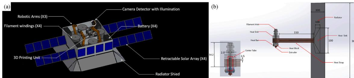
Fig. 11. (a)FDM concept for in-space manufacturing,(b) extruder and thermal unit structure [95].
