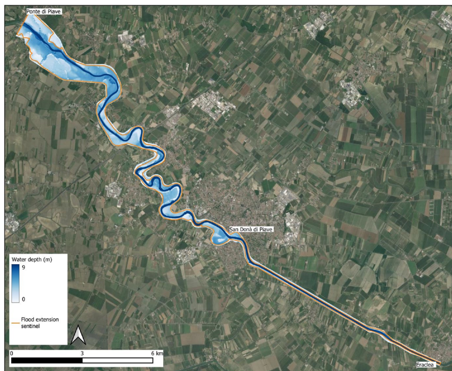
Fig. 11 Flood extent and water depths simulated at the time of the satellite image. The orange polygon outlines the flood extension observed in the satellite image
