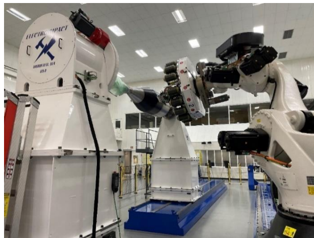
Figure 4. Test article being manufactured with the MSFC AFP robot.
