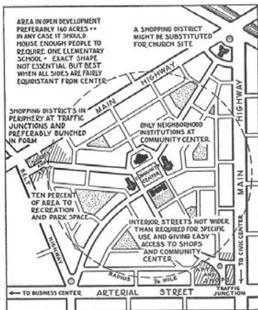
Fig. 3. Clarence Perry, Neighbourhood Unit, 1928. New York Regional Survey, vol.7, 1929 This diagram clearly shows and explains Perry's intended hierarchy for urban space.
