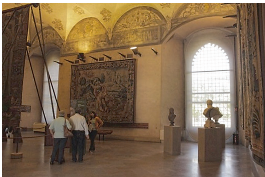
Fig. 10.4 The current experimental installation of two screens at Sala del Gonfalone, Castello Sforzesco. The textile panels tested on the two windows are experimenting different degrees of density, air permeability and translucency to the natural light (Zanelli et al. 2020)
