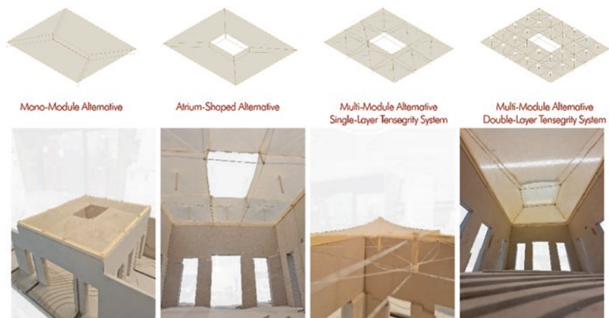
Fig. 10.8 Design alternatives of double-layer tensile canopies
