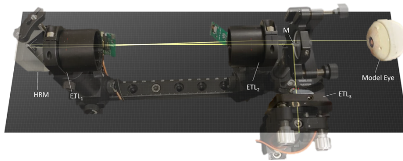
Fig. 5. Overlay of a picture of the experimental beam scanner prototype with the ray tracing of the beam through the beam scanner for the starting position of the anterior segment scan configuration. Visualization 2 shows the sequence of eight discrete positions for the anterior and posterior scan configurations.
