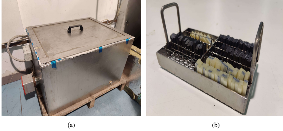
Figure 3: Conditioning chamber (a) and specimens holder (b)
