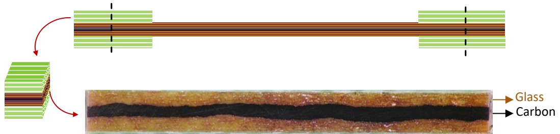
Fig. 6 Variation of thickness over the cross-section of the specimen with continuous tabs.
