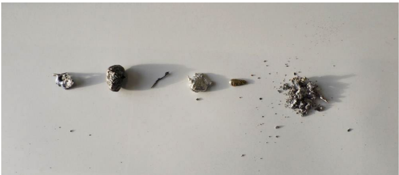
Figure 2: Some of the metals recovered from an old MacBook Pro melted and casted. Still image from a video. Credits: authors
