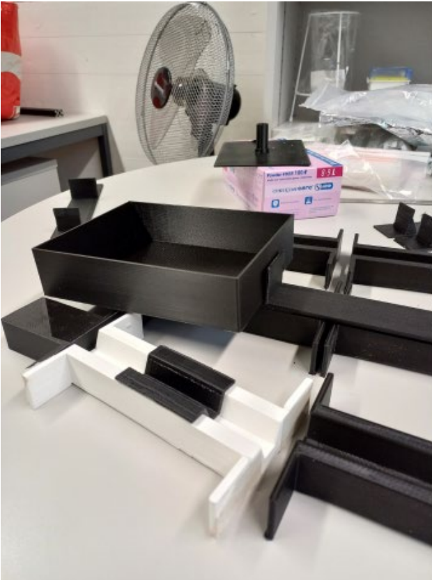
Figure 12: Mock-ups used to simulate the automation system of the swab trays: on the left elements before assembling, on the right same elements in the prototyping setting.
