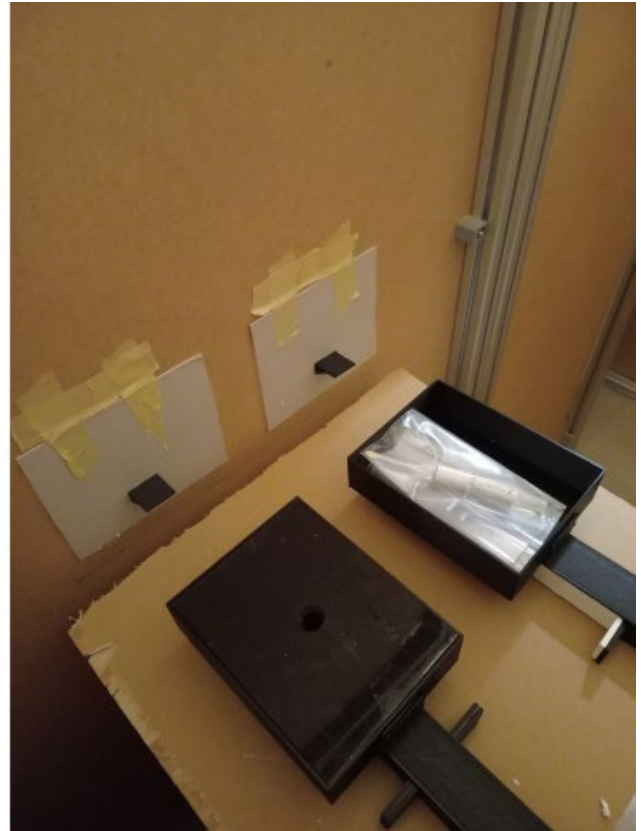
Figure 12: Mock-ups used to simulate the automation system of the swab trays: on the left elements before assembling, on the right same elements in the prototyping setting.
