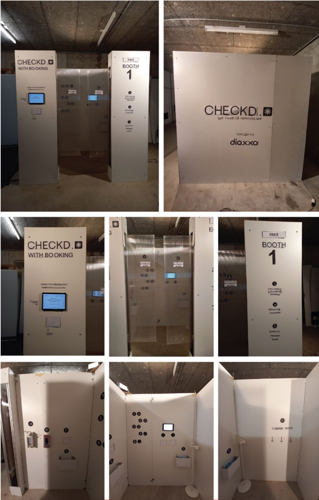
Figure 13: The Checkd. Booth 1:1 scale prototype. In order: front and back, zoom on front (check in interface, doors, information panel), interior left wall (hand sanitization, saliva generation slot), interior centre wall (signage, procedure interface, sample slots), interior right wall (luggage area).
