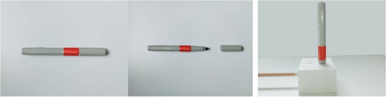
Figure 7: The tool used in procedure #1 to simulate a swab having the same concept of a marker, the red tape signaled a "no-touch" zone.
