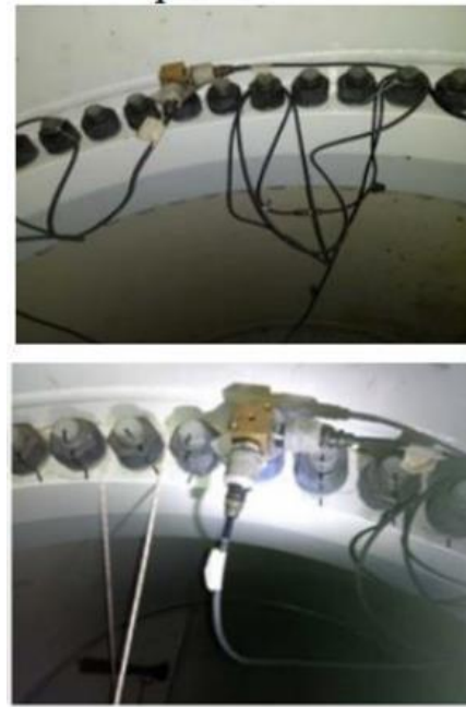
Figure 4 Detail of the installed Accelerometers
