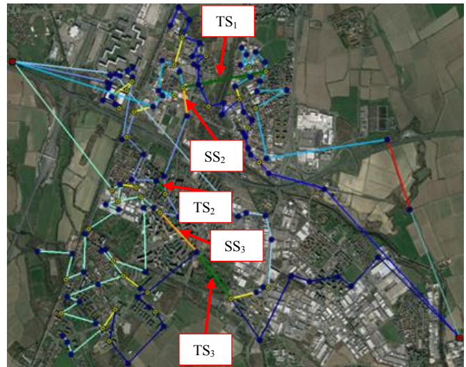
Figure 9. Best feasible solution. The green color indicates the closure of a previously open switch (TS); the orange color the opening of a previously closed switch (SS).
