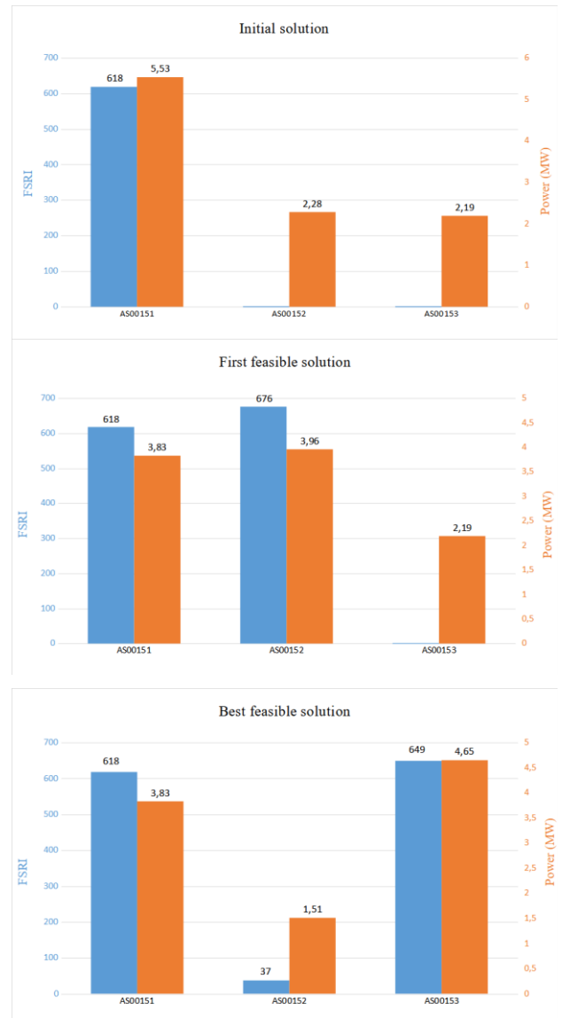
Figure 11. FSRI and power flowing on the related feeder for the initial solution, the first feasible and the best feasible solutions.
