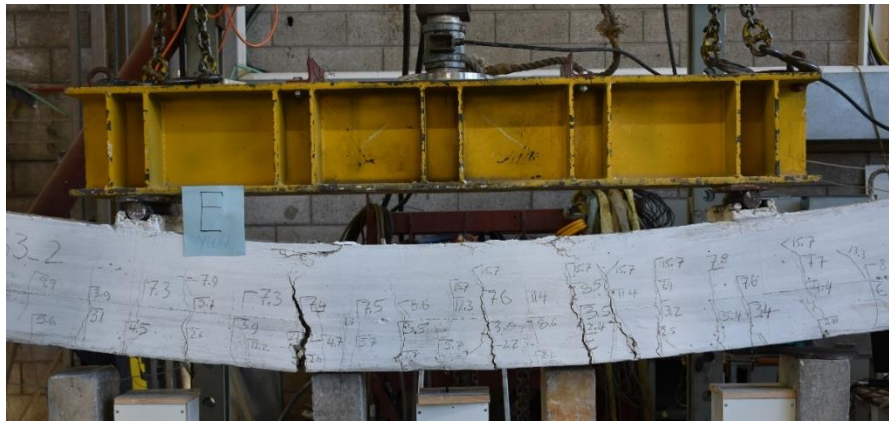
(b) Several wide cracks
