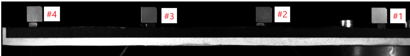
Fig. 13. Aluminum beam and accelerometers used for the experiments.
