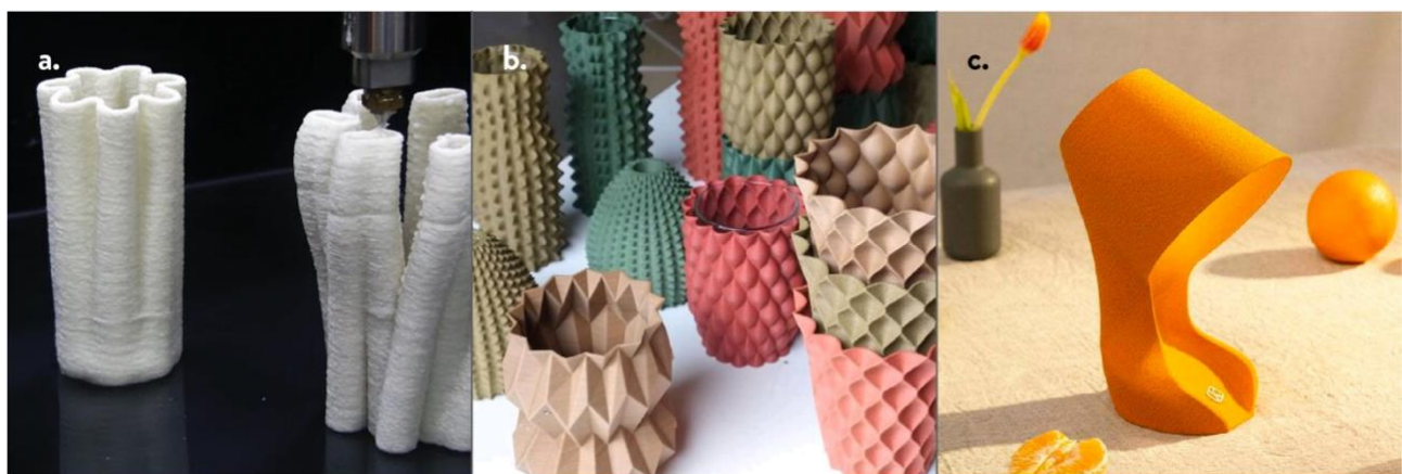
Fig. 8. Examples of 3D printed applications from biomass waste: (a) “Natural Composite Pillar” made of chitin/cellulose composite through large format DIW [68]; (b) “Hemprinted” e-shop of products and filaments for FFF made of PLA filled with hemp, tomato, and pomegranate waste [103]; (c) “Ohmie Lamp” made of PHB filled with orange peels through FFF by Krill Design [105].
