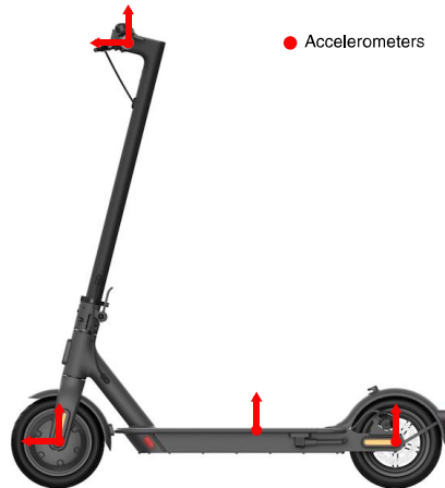
Figure 3. Experimental setup: location of accelerometers for the acquisition of accelerations when passing over a lumped obstacle
