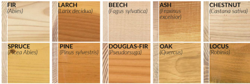
Fig. 2.2 Wood species for construction uses. Source Author's elaboration on illustrations retrieved from [19]
