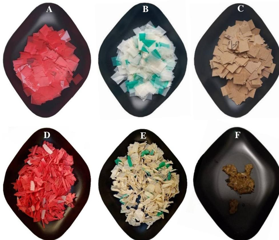
429 Figure 4 Pieces fed to semi-continuous tests of BSB1 (A), BDB1 (B), and PB (C). Undigested pieces of semi-continuous 430 tests washed and dried of BSB1 (D) and BDB1 (E). Undigested pieces of semi-continuous tests of PB (F).
