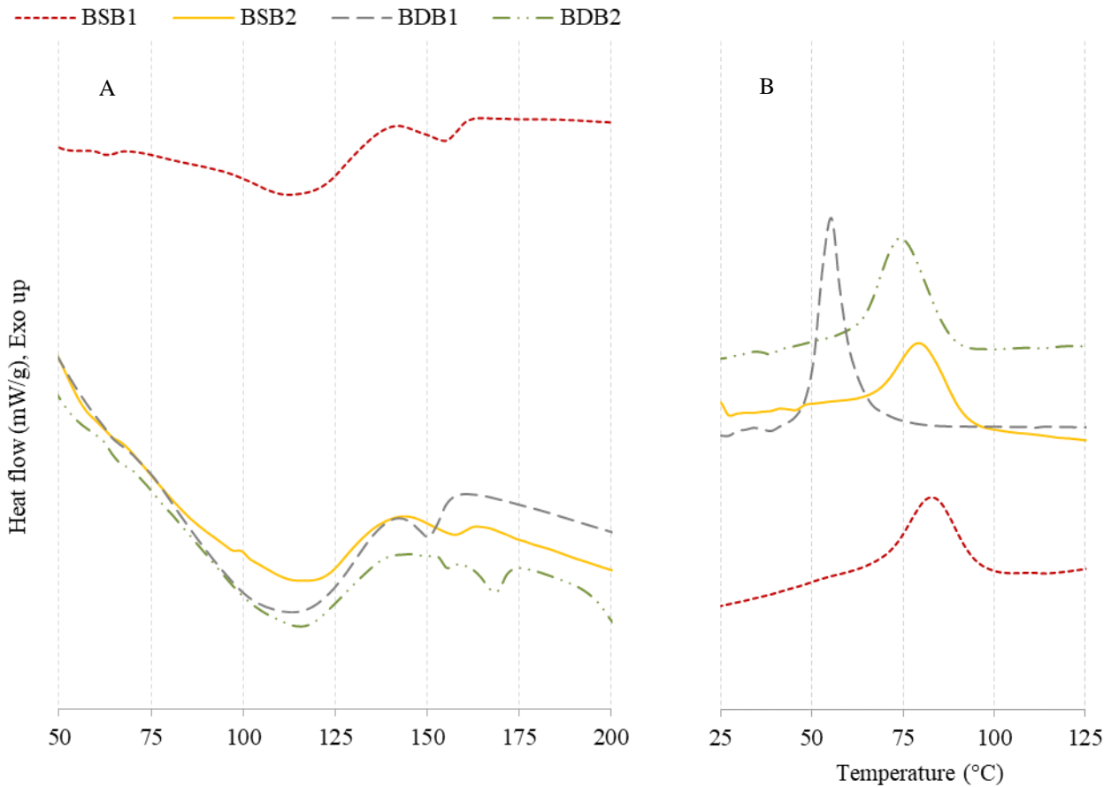
305 Figure 1 DSC thermograms of melting (A) and crystallisation (B) of tested bioplastic bags.
