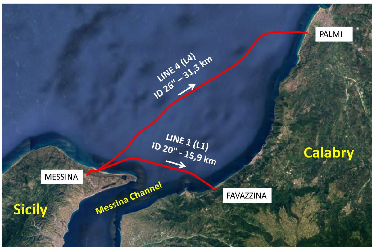
Figure 1. Messina channel subsea natural gas transportation pipelines. In red the tracks of LINE 1 (15.9 km length, internal diameter ID=20") and LINE 4 (31.3 km length, internal diameter ID=26").
