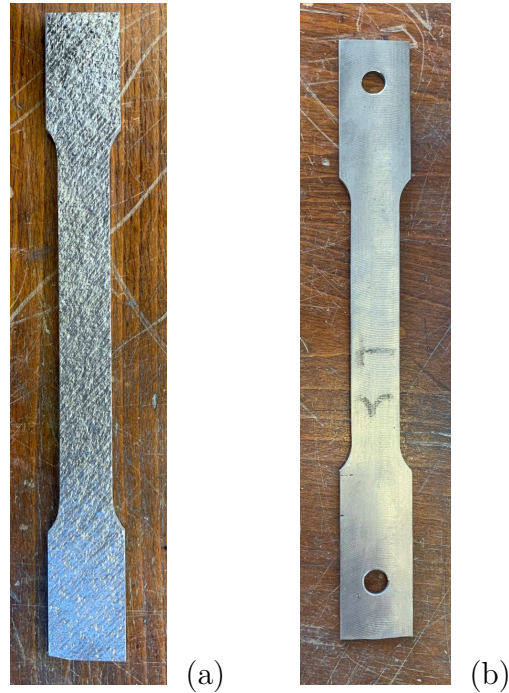
Figure 3: Surface roughness of the dog-bone specimens: as cut from the as-built plate (a), after surface milling (b) [16, 18, 43].
