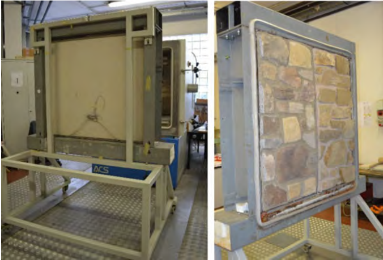
Fig. 2 Views of “door” sample in front of the climatic chamber before the sensor wiring
