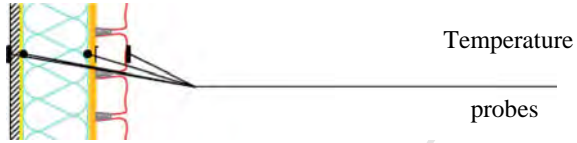
Fig. 1 Temperature probe positioning
