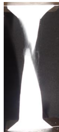
Image of the sample breaking (aligned fibers)
