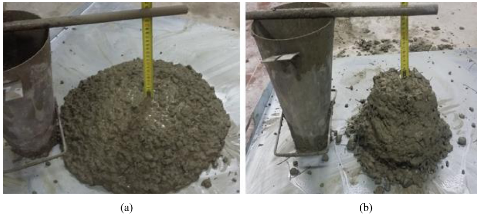
Fig. 1. Appearance of fresh concrete in slump test: (a) plain concrete and (b) concrete reinforced with 1% DHE steel fiber.
